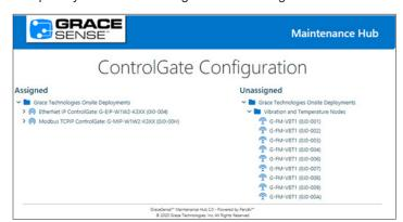
This case has one EtherNet/IP™ ControlGate™ and one Modbus TCP/IP ControlGate™ and 9 Vibration and Temperature Nodes. Your screen will vary in quantity of nodes and names used.
