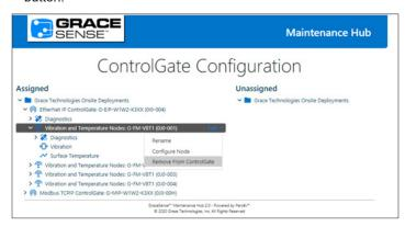
8. Once complete, your node tree will look something like the below. In this case, Nodes 0J0-001 through 0J0-004 were assigned to the EtherNet/IP™ ControlGate™ 0I0-004. Nodes 0J0-006 through 0J0-00A were assigned to the Modbus TCP/ IP ControlGate™ 0J0-00H. All nodes were assigned so the Unassigned column is empty.
