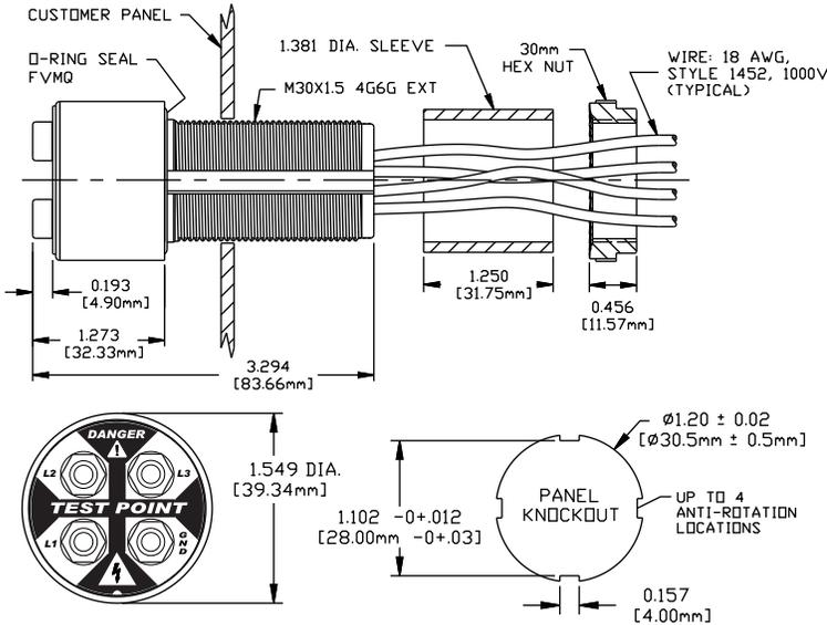
NOTE: (4) Test point jacks accept .080" DIA. probe points.
