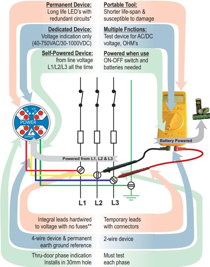
**Warning:** Before working on an electrical conductor, verify zero electrical energy with proper voltage testing instrument and the proper procedure as per NFPA 70E 120.1(5), 120.2 (F)(2)(f)(1-6), OSHA 1910.333(b)(2)(iv)(B).
