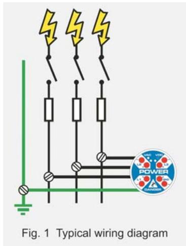
Understanding how VIs function helps clarify many application questions that arise when applying this device into any type of power system. Most examples will use a 480VAC 3-Phase system (Fig. 1).
