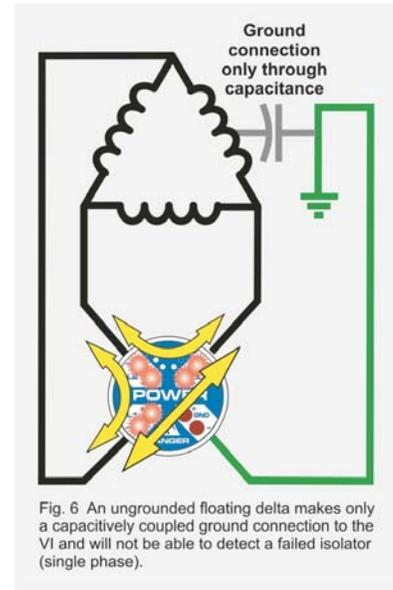
Fig. 6 An ungrounded floating delta makes only a capacitively coupled ground connection to the VI and will not be able to detect a failed isolator (single phase).
