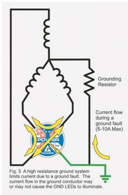
Fig. 5 A high resistance ground system limits current due to a ground fault. The current flow in the ground conductor may or may not cause the GND LEDs to illuminate.
