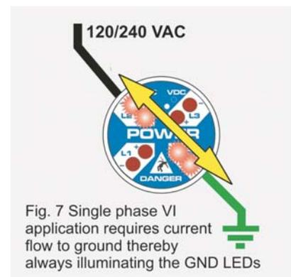
Fig. 7 Single phase VI application requires current flow to ground thereby always illuminating the GND LEDs
